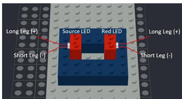
For each LED, make sure you know which of the pins is the longer one. **Separate the legs** of the LEDs to ensure they won't touch and short the circuit.
