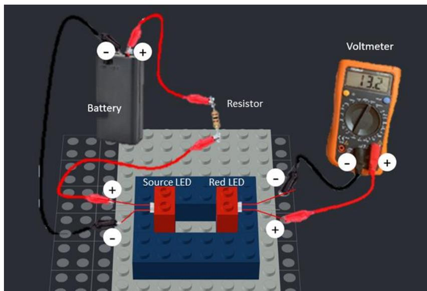
Turn the multimeter to the  $2000m$  (2000 mV) direct voltage setting. If the source LED is lit up, this should produce a non-zero reading of roughly 600 – 1000 mV. You should also be able to observe that the voltage reading drops if something, such as a finger, is inserted to obstruct the light path between the two LEDs.
